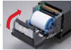
4. Close front door to complete the auto paper loading
